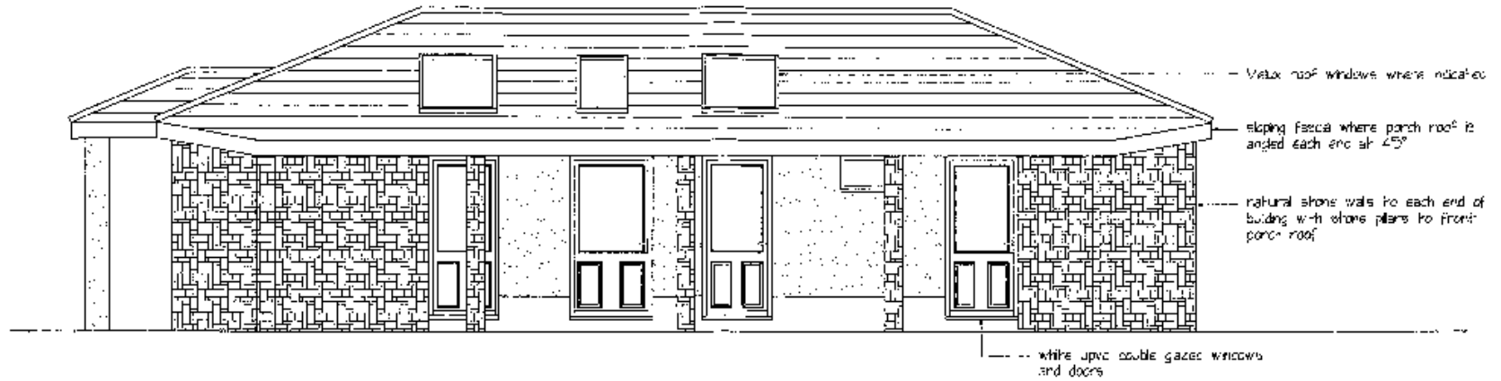
Proposed front elevation Scale 1:50
